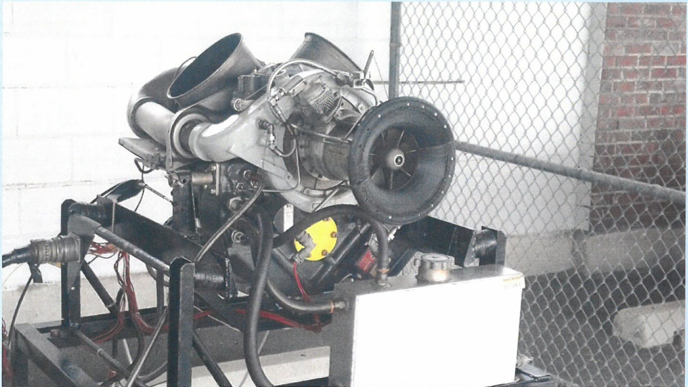
Figure 7. Turbine engine test run with 3D printed inlet installed.
