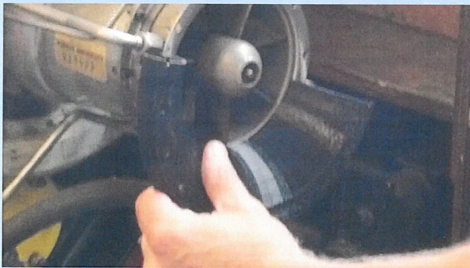
Figure 6. 3D printed bellmouth inlet installation.
